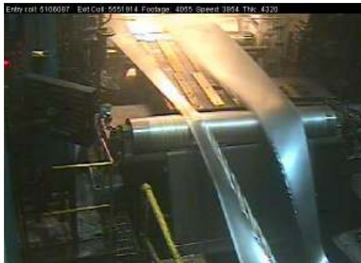
Figure 5 – Coil breaks entering the mill
