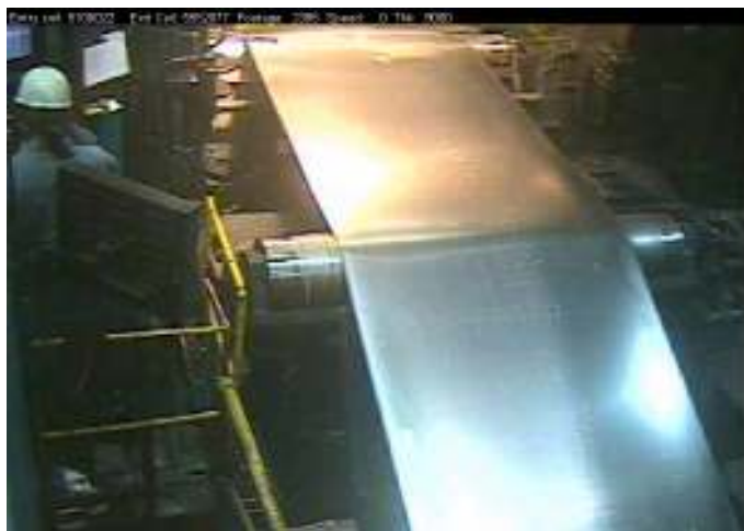
Figure 3 - Roller failed to detect the defect, but upon reviewing, the coil image quality inspector identified it
