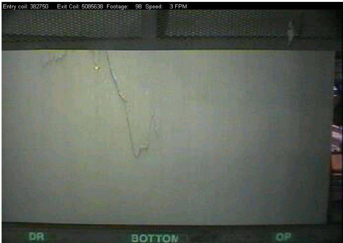
Figure 9 - The image of the suspected coil was reviewed and the exact location of the defect was found
