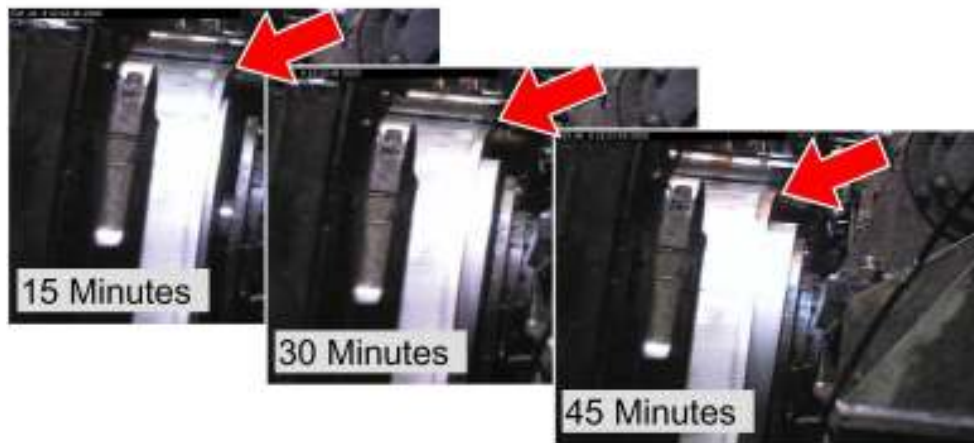
Figure 17 – Uncoiler drifts forward causing coil to loosen and telescope.
