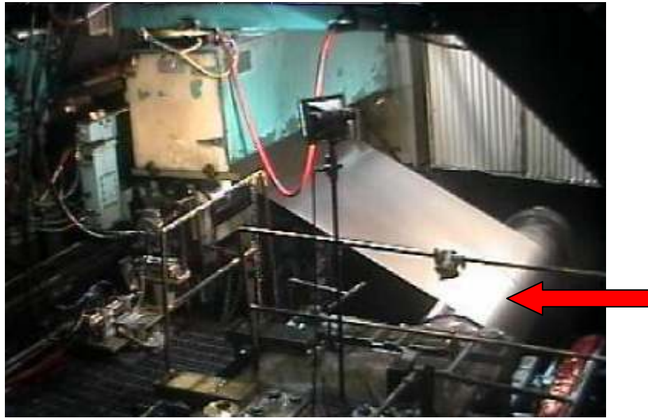
Figure 6 – Mill backed up after belt wrapper came in causing crease that carried through entire coil
