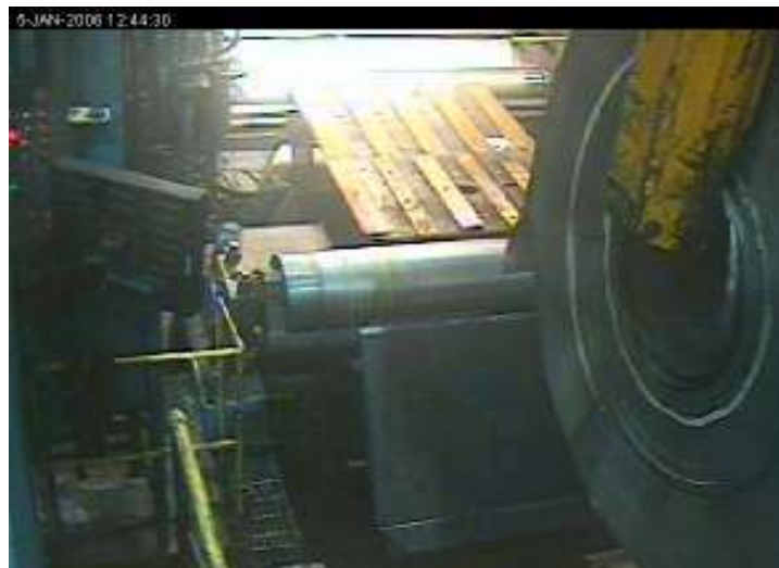
Figure 4 – Coil is chalk-marked with winding problem as it is loaded
