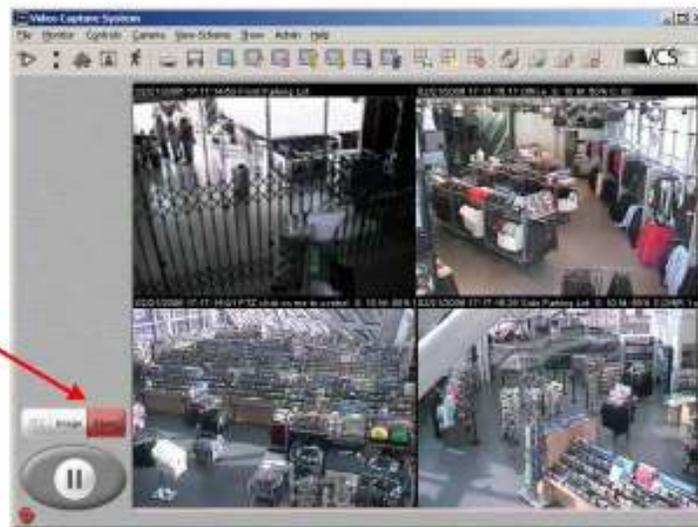
When the Alert button is clicked on, the Live screen will change to a Review screen with a list of alarms being displayed on the left part of the following screen (highlighted in red). The “Disable Alarms” are used for a temporary period when the exhibit areas are cleaned or changed.
